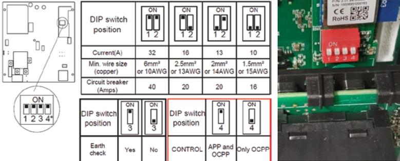
Figure 9 DIP Switch Positions
