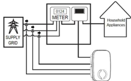
Figure 14 three-Phase System CT Clamp Positioning
