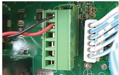
Figure 19 Incorrect Connection
