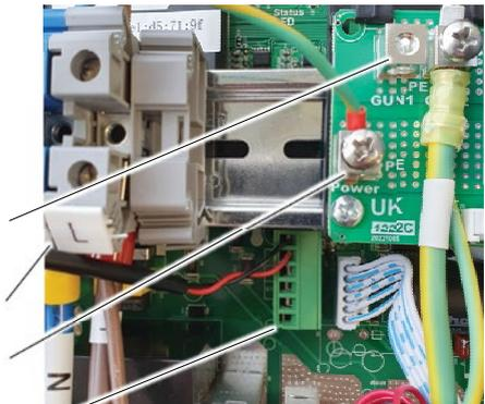
Figure 18 CT Connector Block
