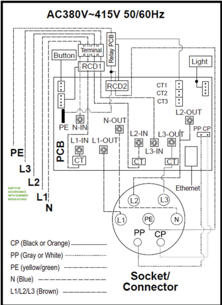
Figure 7 EVON00100 - 3-Phase, Version Schematic Diagram
