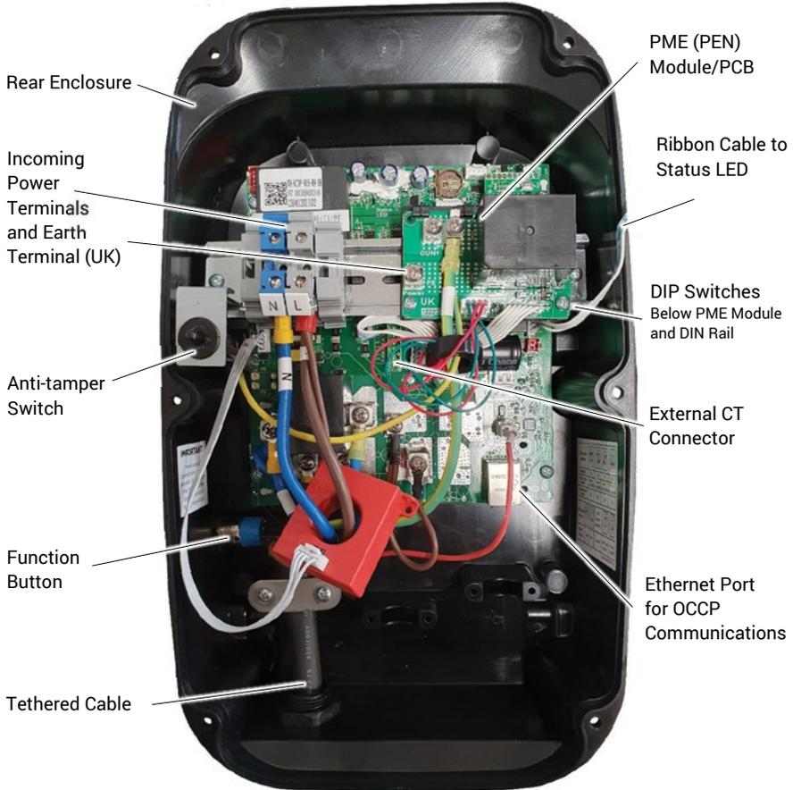
Figure 2 Internal Arrangement (1-phase, Tethered model shown)
