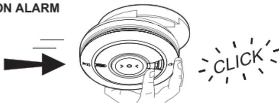
SLIDE ALARM ONTO BASEPLATE. A CLICK SHOULD BE HEARD AS THE TAMPER-PROOF CATCH ENGAGES
