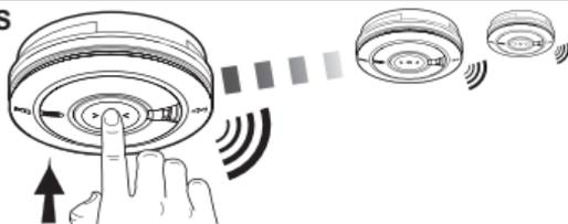
PRESS AND HOLD THE TEST BUTTON ON THE ALARM. THE ALARM AND ANY OTHER INTERCONNECTED UNITS SHOULD SOUND
