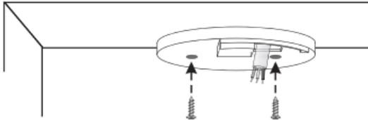
WIRE TO TERMINALS ON THE BASEPLATE AND FIX BASEPLATE TO CEILING USING THE FIXINGS PROVIDED
