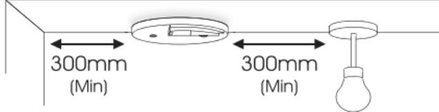
ALARM SHOULD BE CEILING MOUNTED AT LEAST 300mm FROM WALLS & OBSTRUCTIONS, IDEALLY CENTRALLY IN ROOM/AREA
