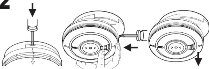
WITH THE SCREWDRIVER STILL INSERTED, PUSH THE LOWER HALF OF THE ALARM AWAY FROM THE SCREWDRIVER, IN THE DIRECTION OF THE ARROW ON THE COVER
