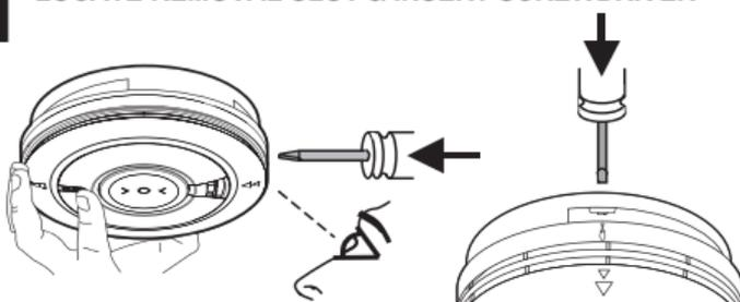
LOCATE THE ARROW ON THE FRONT FACE OF THE ALARM
